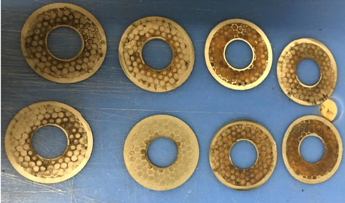
Picture showing impurities removed from steam flow on stainless steel media.
