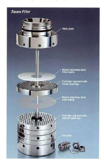
The patented segmented construction of MICROPURE filters offers significant advantages over conventional cartridge filters (shown above). Steam flows into the openings on the outside of each segment disc and passes through the filter and into an adjacent disc. Filtered steam exits through the opening at the center of the cartridge, free from contaminants that can affect the quality of your product.
