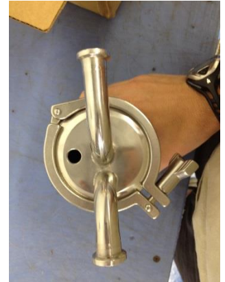
Picture of Drain Port on base of housing. A single drain valve or plug can be installed. Recommendation
