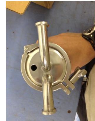
Picture of Drain Port on base of housing. A single drain valve or plug can be installed. Recommendation varies by application.
